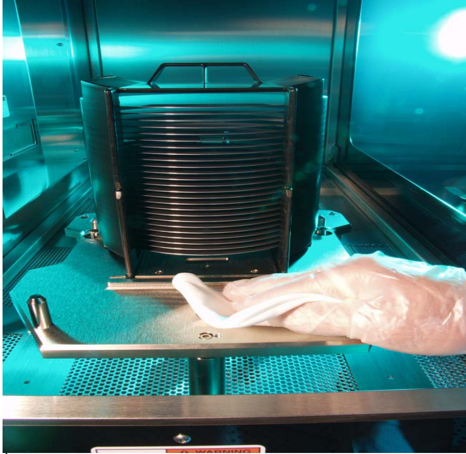
Figure 7. Maintaining cleanliness of wafer loading area is critical
