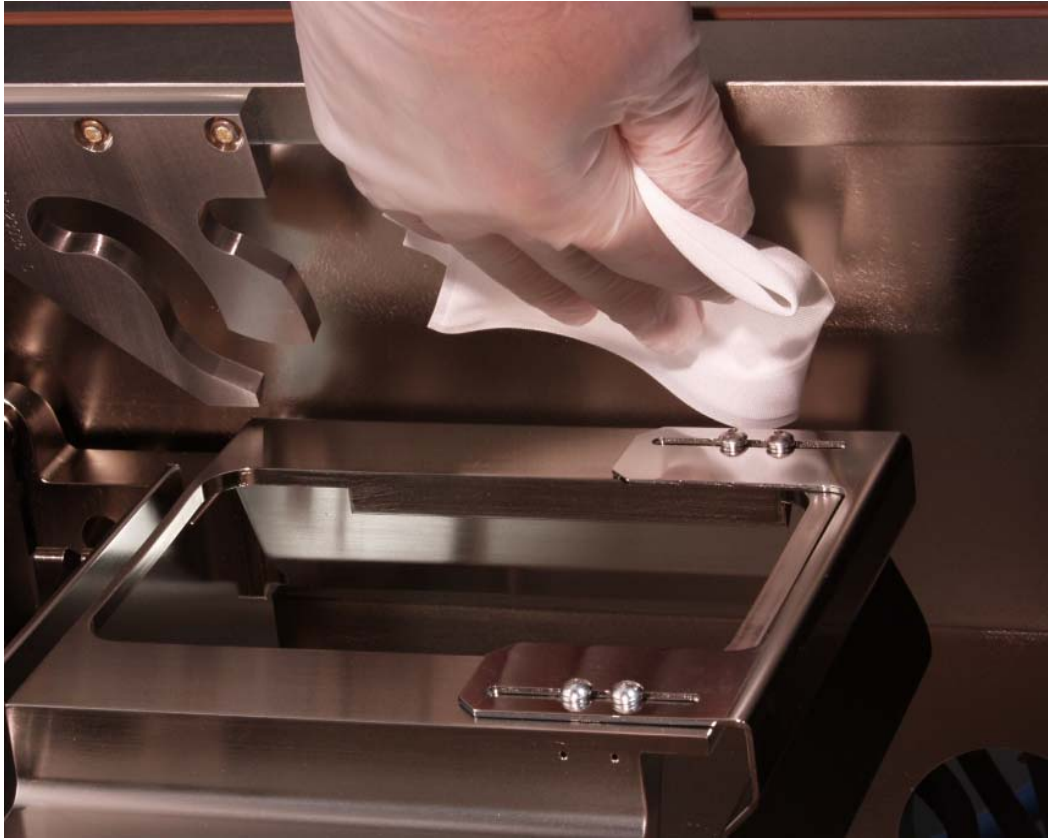
Figure 6. Wipedown of process equipment during preventative maintenance (PM)
