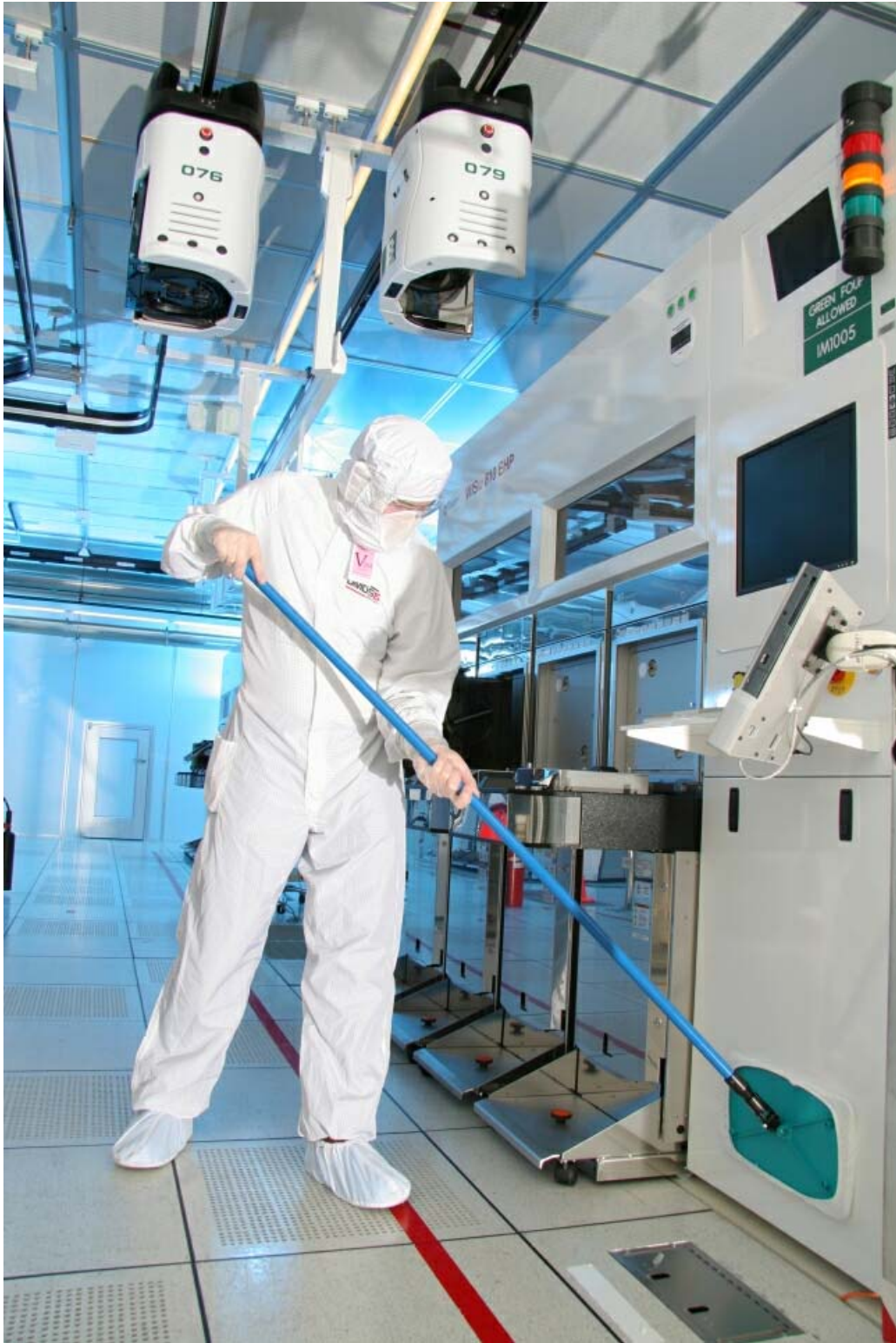
Figure 5. – Wipdown of equipment exteriors in 300 mm fab
